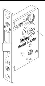
2. Place turnpiece plate over barrel, onto the door surface, so that plate is aligned with the center of the turnpiece hub in lock.
