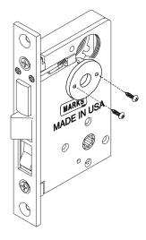
3. Mark screw holes of the plate and fasten to door. Then remove alignment tool.
