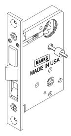
1. Insert shaft of alignment tool into turnpiece hub of mortise lock so barrel of tool reaches the door surface.
