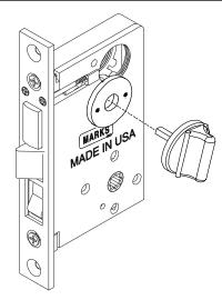
4. Insert spindle of turnpiece assembly into turnpiece hub and fasten the turnpiece rosette to the turnpiece plate.
